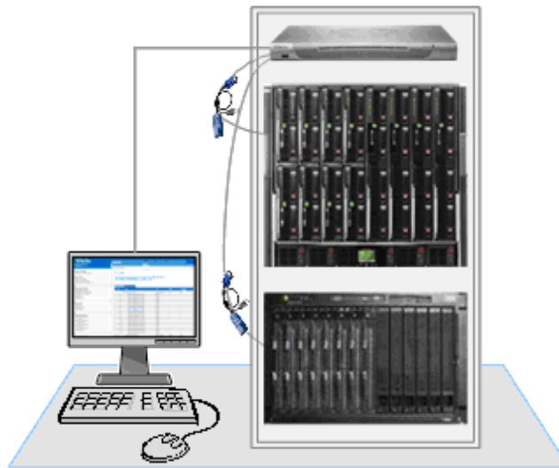
Figure 1. Dominion KX II provides out-of-band access to blade servers by physically connecting a Computer Interface Module to the blade chassis.
